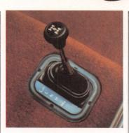
drive. "H-LOC" locks out the inter-axle and connects both front and rear axles while operating in direct drive. It is used when low traction surfaces could cause wheel slippage. With Full-Time four-wheel drive, included in conjunction with available automatic transmission and V8 engine, you enjoy balanced driving power and traction effort at all four wheels. GMC
